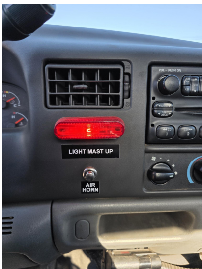
Mast Warning Light #1 is located in the truck's cab to the right of the steering wheel.
