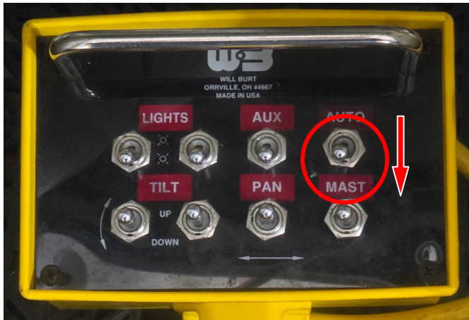
Figure 5.1 - Option A Toggle mast switch down
