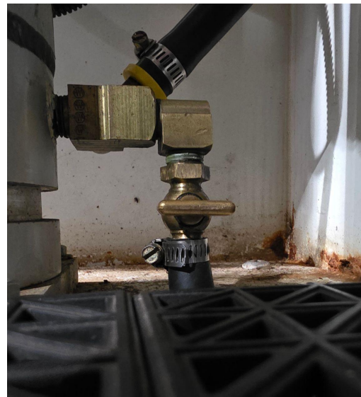
Figure 3.5 - Horizontal Valve When the valve is horizontal, it is closed . This is the position it should be in when the mast needs to go up and be in operation.
