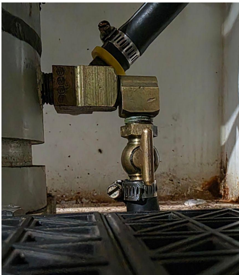
Figure 3.4 - Vertical Valve When the valve is vertical, it is open . Air will release and the mast will descend. This is the position it should be in when the mast is not in use.
